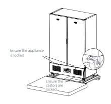
Support the appliance on the front, cut the support straps on both sides and rear then unlock the castors.
