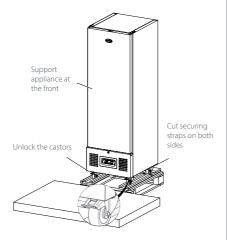
5 Carefully slide the appliance off the pallet onto the adjacent level surface.
