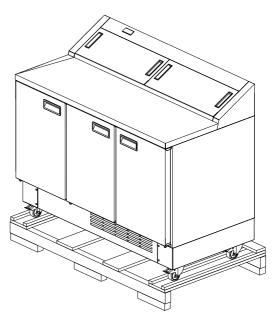
**3** Ensure that castors are locked and the doors are taped closed to prevent opening.
