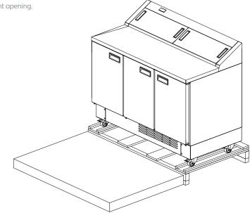
**4** Support the appliance on the front, cut the support straps on both sides and rear then unlock the castors.
