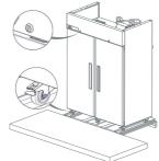
4 Support the appliance on the front/top of the door and rear as the appliance is top heavy, cut the support straps on both sides and unlock the castors.
