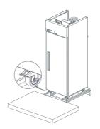
5 Carefully slide the appliance off the pallet onto the adjacent level surface.
