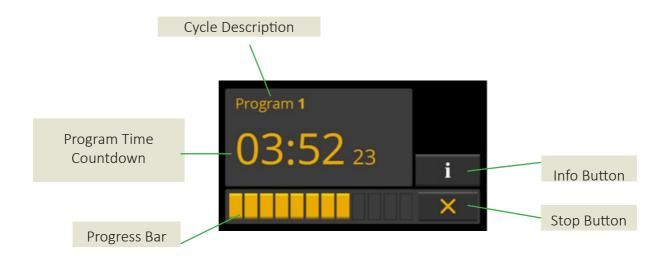
In order to provide a highly visible, readily understandable format for the operator, the display screen uses a 'surround signal'; a colour code that has phase specific meanings as follows:
