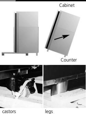
**Important (Cabinets only):** Ensure a minimum clearance of 150mm above unit and ventilation for efficient operation. Where possible, ensure the unit is not adjacent to a heat source.
