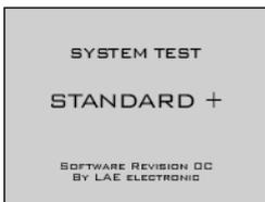
When mains electrical power is first applied to the controller it will carry out a self-test function, for approximately 3 seconds. During this period the display will show.
