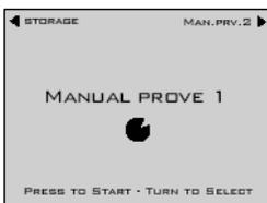
On completion of the self-test, the controller will revert to the last chill program that was run Storage, Manual Prove 1, Manual Prove 2, Manual Prove 3, ADPR 1.
