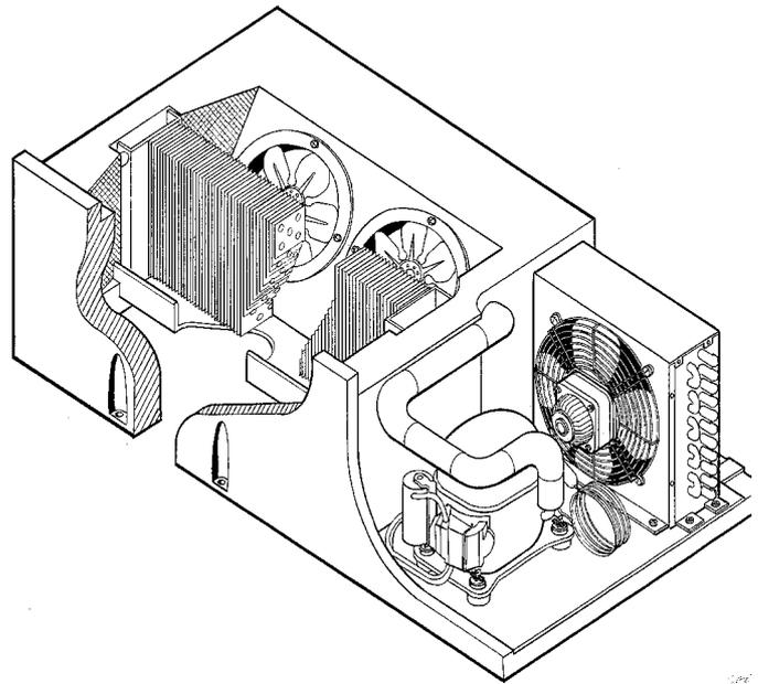
Fig 4B Double Section Plug Box
