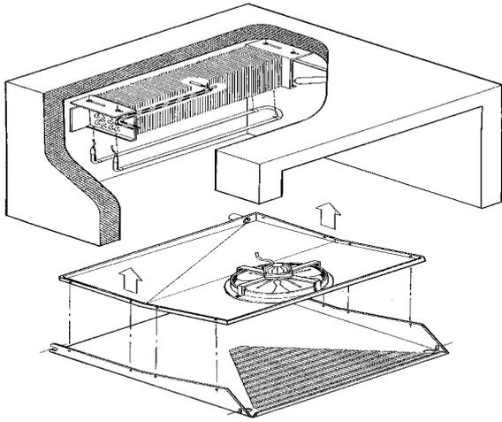
Fig 7A. Single Section Evaporator Housing.
