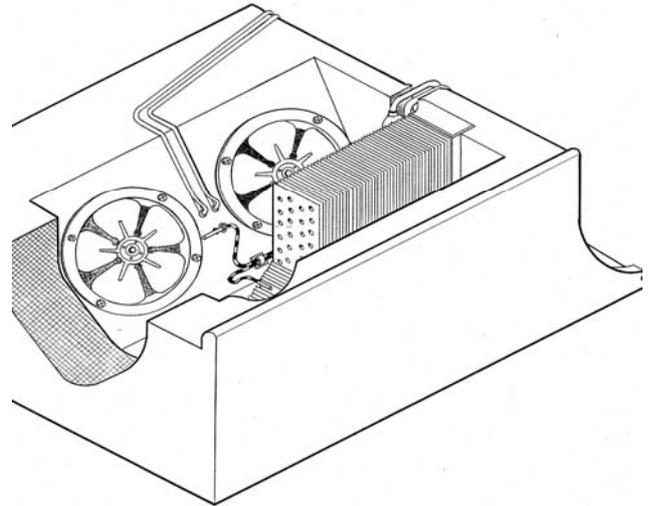
Fig 6B Double Section Top Mount.
