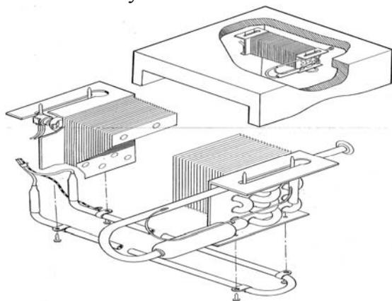
Fig 9A. Single section Evaporator
