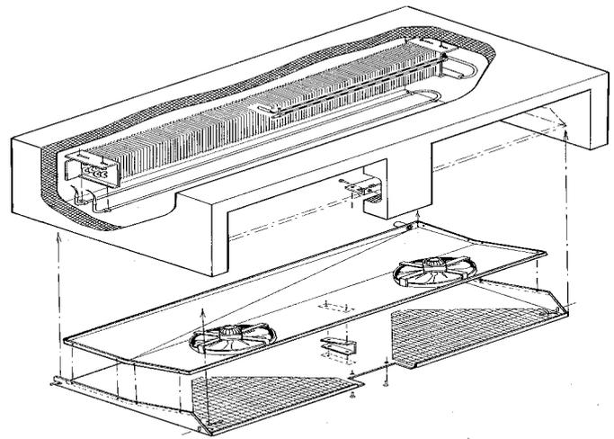
Fig 7B. Double Section Evaporator Housing.
