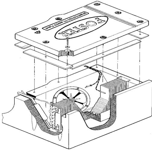
Fig 6A Single Section Top Mount.
