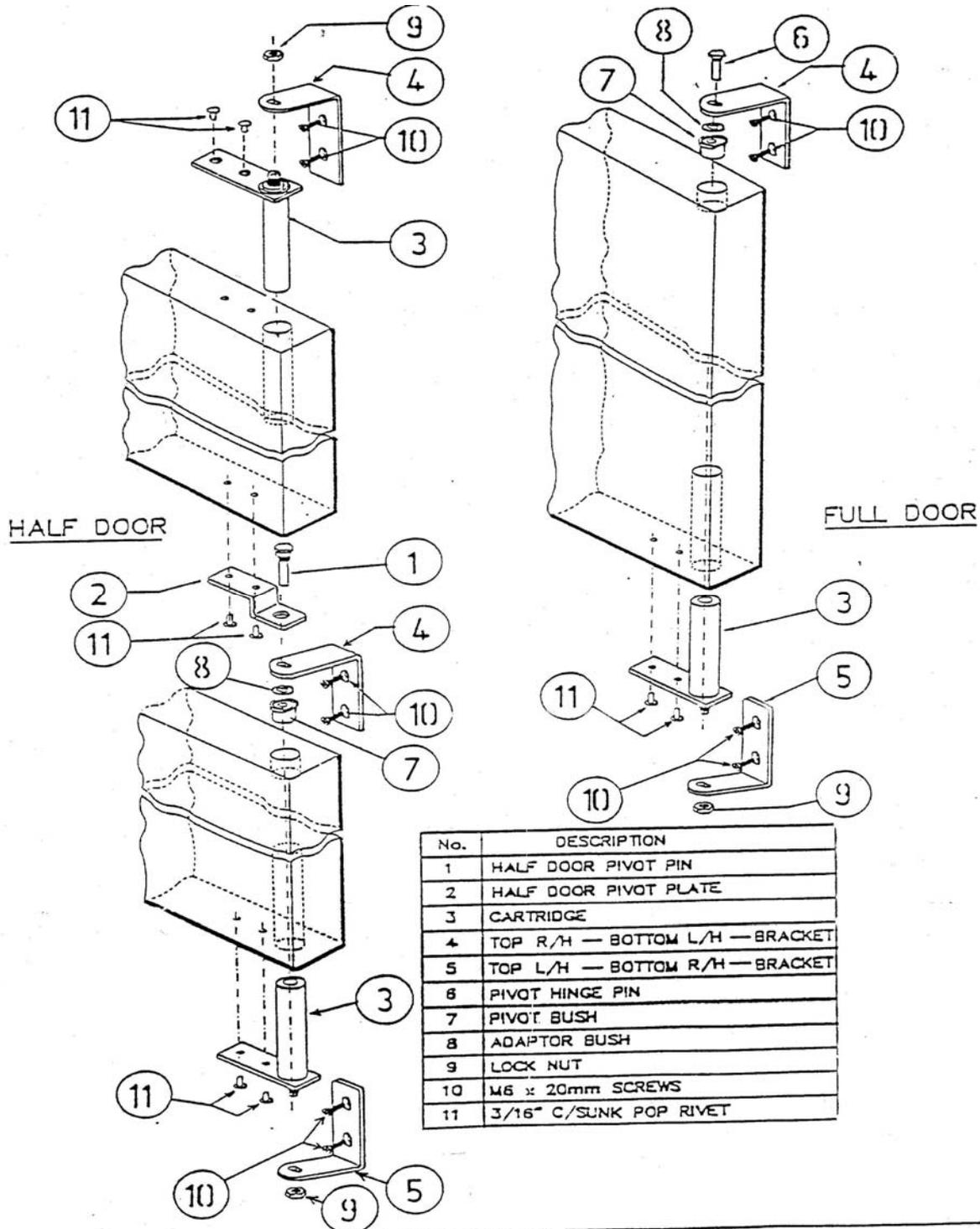
Fig 11. Standard Hinge Parts.
