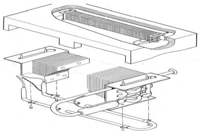
Fig 9B Double section Evaporator
