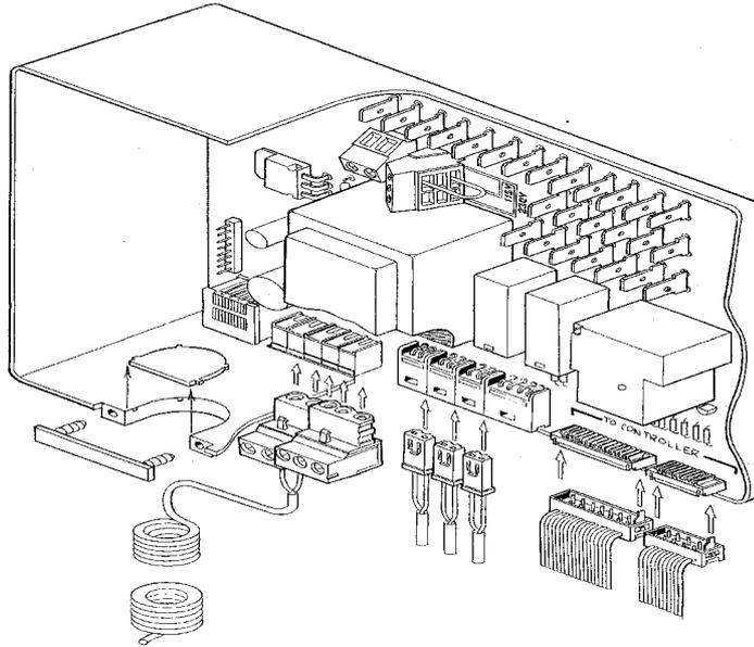
Fig 1. Power Switching Unit.
