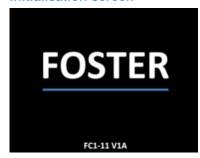
After power is applied to the unit the controller display will show the initialisation screen. This will only show for a few minutes stating both 'Booting' and then displaying the software version at the bottom of the screen. When the controller has completed initialisation the screen will revert to the 'Home Screen'.
