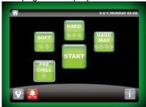
To view this alarm and or the alarm history press the flashing red alarm bell (as seen above) or if the alarm has been rectified access this history screen by navigating through he 'Service Settings' Screen and selecting Alarms.
