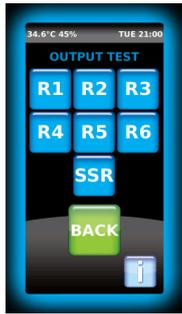
This function is a useful tool that will aid engineers in basic service diagnostics. When 'Relay Test' is selected from the 'Service Settings' screen the engineer can select each relay individually to energise the linked part. During testing the relay selected will highlight the block in blue and unless manually switched off (by pressing the relay number again) will run for 2 minutes before de-energising. More than one relay can be activated at a time.
