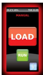
**Load Alarm** – press the green 'Run' button to continue the cycle and confirm product has been loaded into the unit
