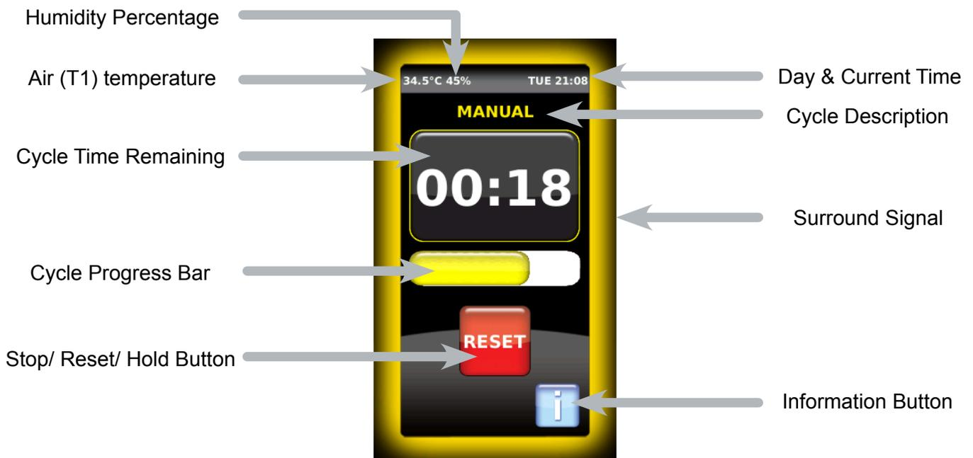
*(Some icons or switches are only visible during adjustment, when activated by parameters or through operation/manual selection).*
