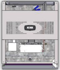
2. Remove the self-tapping screws that retain the unit cover and top surround with a screw driver.
