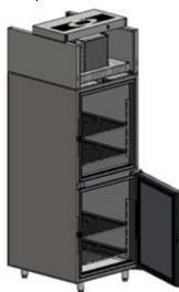
5. Remove the middle hinge bracket and remove the bottom door.
