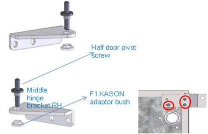
7. Fit the bottom door and top hinge bracket
