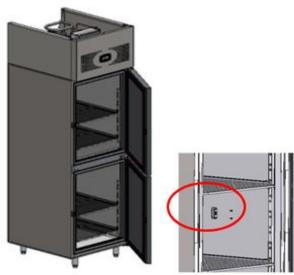
3. Remove the unit cover and lay on the top of the unit. **DO NOT disconnect any wiring.**
