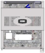
5. Remove the bottom hinge screws and bracket re-assemble the bracket on the opposite side (as shown). Fix the bottom hinge bracket assembly in the correct position on the cabinets bottom clad.
