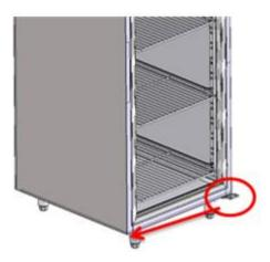
6. Rotate the door 180 degrees and install on the bottom hinge bracket. Locate the top hinge bracket on the door cartridge and the fix the top hinge bracket to the cabinet shell. (See screw positioning images below)
