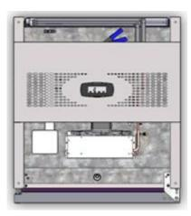
2. Remove the self-tapping screw that retains the unit cover and top surroud using a screw driver.
