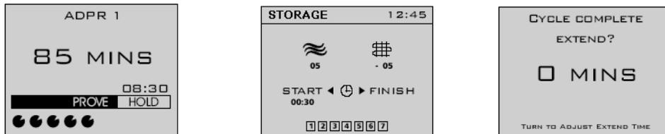
The screen will change to display the unit in 'RETARDING' mode, below left, with the temperature being displayed and 'HOLD' highlighted. The refrigeration system will lower the temperature until it reaches the storage setpoint when the screen will change to display 'STORAGE', below right. The controller will continue to operate within the storage temperature limits indefinitely initiating a time based defrost at pre-set intervals
