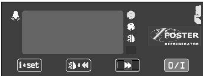
LD1 Controller as used on High temperature Models
