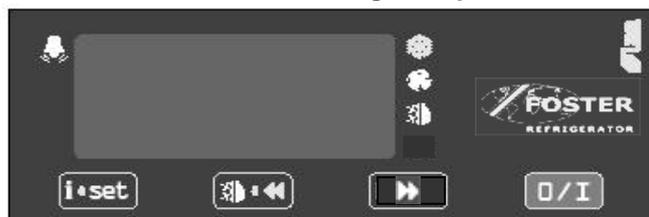
**LD2 Controller as used on Low temperature models**
