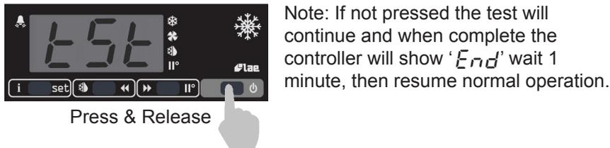
Note: If not pressed the test will continue and when complete the controller will show 'End' wait 1 minute, then resume normal operation.
