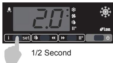
By keeping button **i** pressed, use ◀ and or ▶ buttons to set the desired value (adjustment is within the minimum SPL and the maximum SPH limit)
