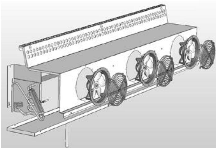
**FPS2HR & FPS3HR Condensing Unit Arrangement.**
