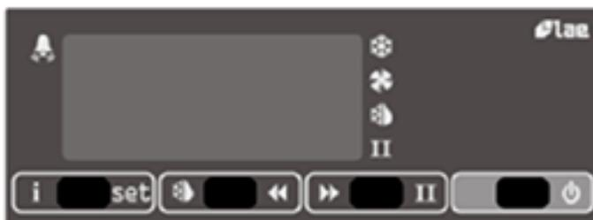
Controller with the LCD 16 Display (00-555740) fitted as from May 2007 to November 2007
