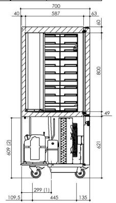
(1) - Evacuation of water from defrost  $\varnothing$ 20 (2) - Electric supply cable
