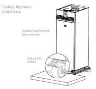
5 Carefully slide the appliance off the pallet onto the adjacent level surface.
