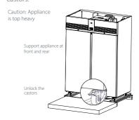
5 Carefully slide the appliance off the pallet onto the adjacent level surface.
