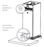
Support the appliance on the front/top of the door and rear as the appliance is top heavy, cut the support straps on both sides and unlock the castors.
