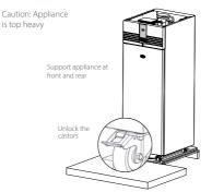
5 Carefully slide the appliance off the pallet onto the adjacent level surface.
