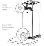
4 Support the appliance on the front/top of the door and rear as the appliance is top heavy, cut the support straps on both sides and unlock the castors.
