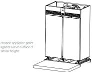
3 Ensure that the castors and appliance door are locked.
